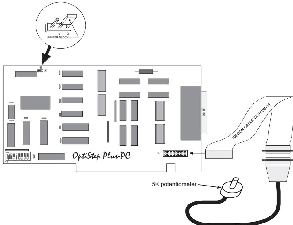
Place the jumper block in the "I" position (between pins 1 and 2) for standard operation.
